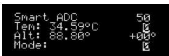
When the highlighted area is on the tilt compensation number(3rd line), the fourth line of the screen displays *Tilt* and the parameters currently being adjusted. Adjust the knob clockwise to increase the number, and rotate the knob counterclockwise to decrease the number.
