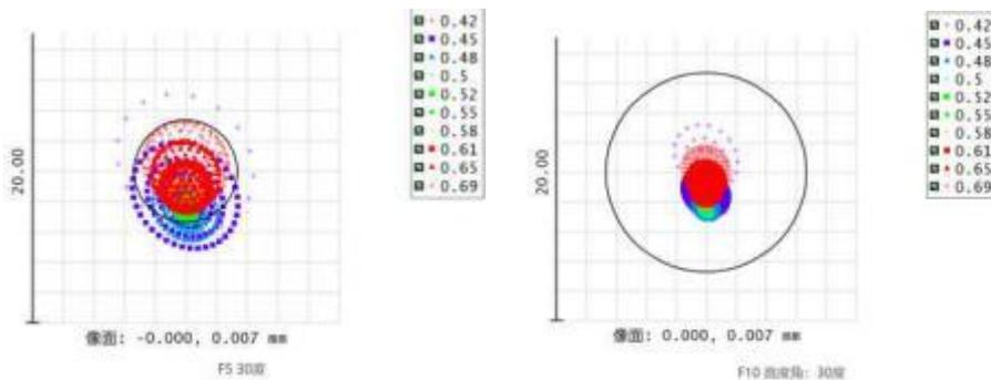
The comparison between spot diagrams of F5 focal ratio (left) and F10 focal ratio (right)
