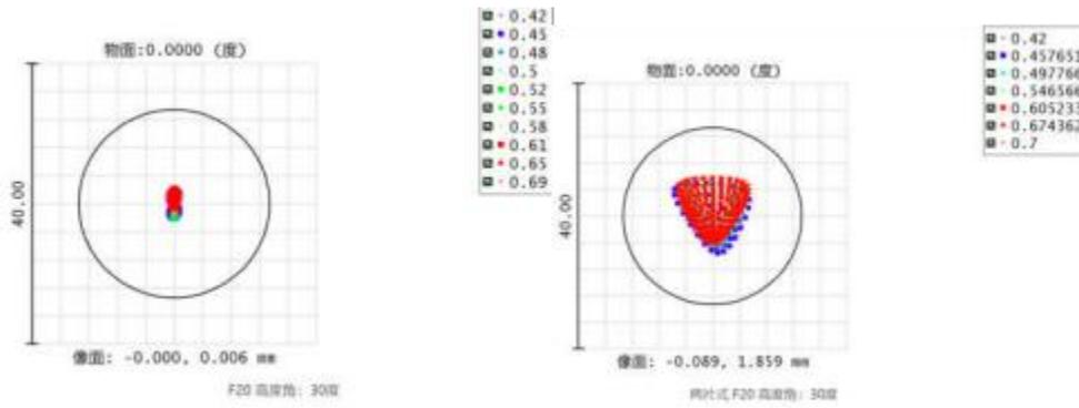
The comparison between spot diagrams of Four-piece None-displacement eADC (left) and traditional Two-piece ADC (right)
