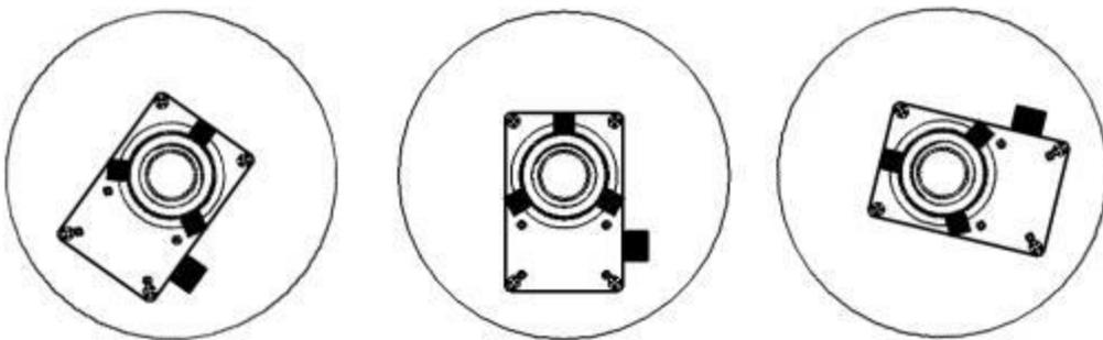
In mode 0, when the eADC optical axis is coaxial with the main mirror optical axis, it can be installed at any angle.
