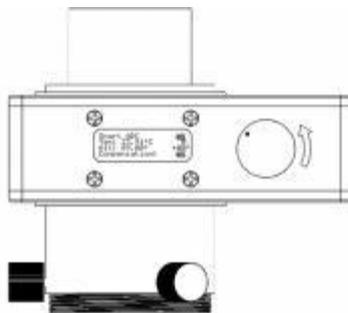
Rotate the encoder clockwise and the highlighted parameter on the display will increase. The setting will be automatically saved 4 seconds later after the adjustment stops. If there is a data change operation within 4 seconds, it will take another 4 seconds to save the data.
