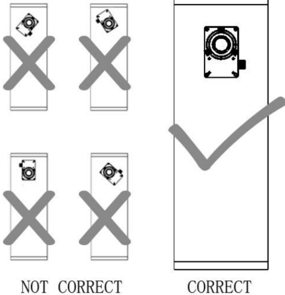
Mode 1: Installation angle diagram of eADC on Newton reflection telescope
