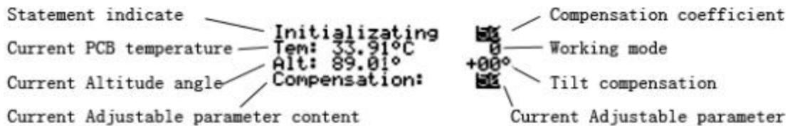
When the highlighted area is on the compensation coefficient number(1st line), the fourth line on the screen displays *Compensation* and the parameters currently being adjusted. Adjust the knob clockwise to increase the number, and rotate the knob counterclockwise to decrease the number.
